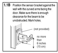
Drill 3/16 inch pilot holes for each sensor bracket and attach the sensor brackets to the wall using lag screws (not provided).
